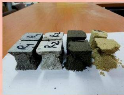
New materials with milled stone content for repairs, tested in the laboratory
