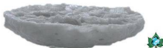
Figure 1: Spongy composite material covered with zinc oxide (MS/ZnO), Patent application no. A/00386/27.06.2019
