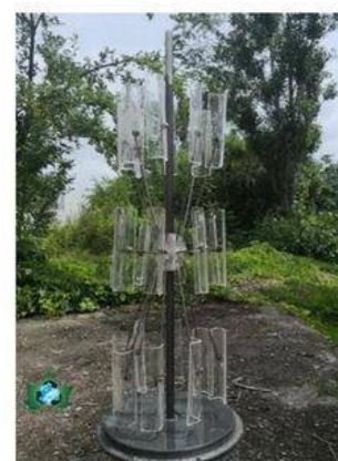
Figure 2: Vertical axis laboratory model with geometry inspired by the bioengineering model of the thistle seed
