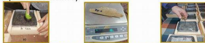
Figure 2. Collecting the exfoliated material, weighing the mass after drying in the dryer, replacing the testing medium with a new one (3% sodium chloride).
