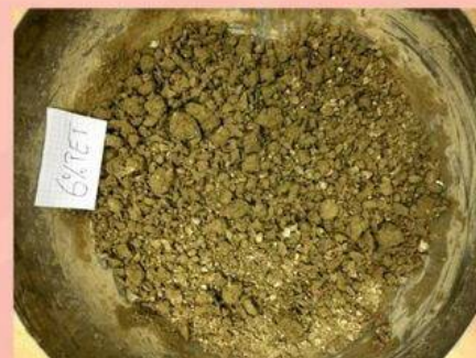
Figure 3. Mixture of clay + 6% PET at optimum water content
