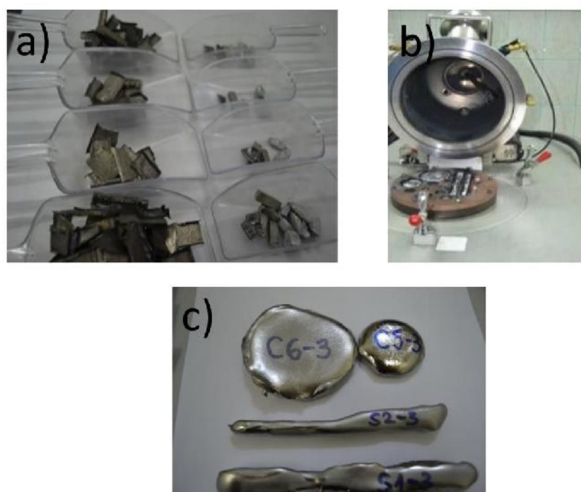
Stages of titanium alloying obtaining process: a) weighing of raw materials and gravimetric dosing; b) loading of the raw material; c) titanium semi-products obtained after solidification
