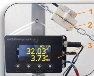
Mini-test bench for the method 1 - Inclinometer; 2 - Support of inclinometer; 3 - Local display mode of the tilt with the output connected to a computer
