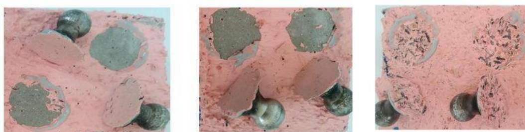
Determination of adhesion to cement mortar surface for RMabb (left), RMacc (middle) and RMadd (right). Type of breaking of the coatings
