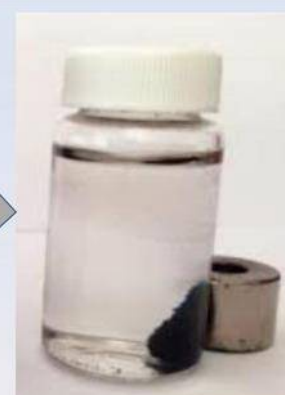
Adsorbent removal using an external magnetic field
