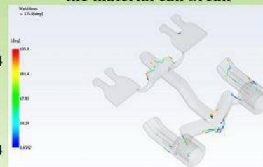
Fig. 18 Places where the breaking of the part may occur
