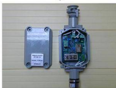
Integrated sensor in H 2 S detector
