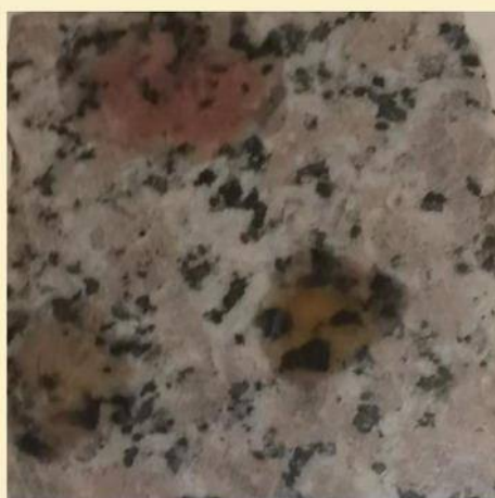
Staining test - granite
