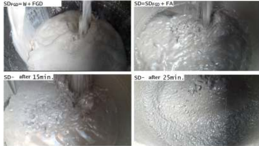
AD=additive; FA=electrofilter fly-ash; SD=dense sludge; FGD=by-product of dry desulphurisation, W=water.
