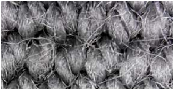
Textile composite obtained by RF oxygen plasma and graphene oxide treatment
