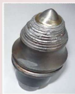
Mill asphalt cutting knife. 1-reinforcement-cutting body with self-protection at wear, 2-knife support made from low alloyed steel with chromium, 3-self-locking when spinning system.
