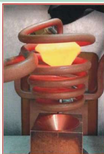
Melting process in levitation.
