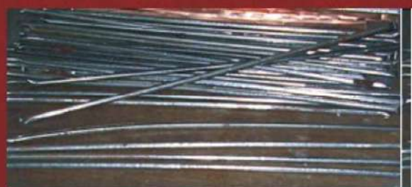
Tubular Rods with Composite Core
