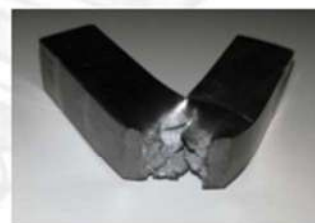
Aspect of high resilient weld
