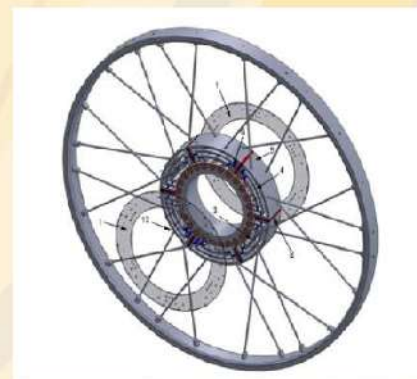
Figure 2. Spatial view of a bike wheel with the electric machine incorporated
