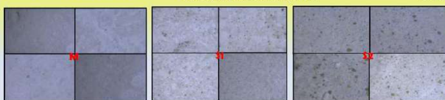
Microscopical aspects on treatment of plaster surfaces; M- untreated; S1/S2- treated with the solutions
