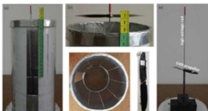
Fig. 3: (a) system overview (b) propeller flight above cylinder (c) top view of the ground cylinder. (d) propeller top view – propeller designed with copper tape (insulated) and two pins per blade. (e) Propeller setup with cylinder removed.
