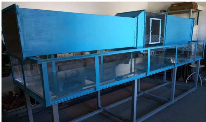
Figure 2: The device for laboratory testing of prototypes of renewable energy production from wind and water sources - foto
