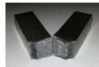
Aspect of non-conform fragile weld
