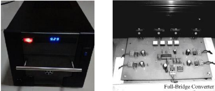
Figure 6. Inverter circuit for ozone tube.
