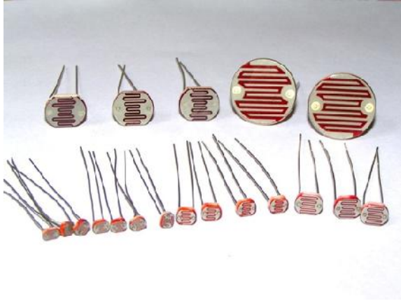
Figure 2. Light dependent resistor [1].
