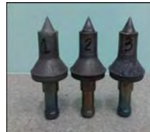
Teeth for asphalt milling having tungsten carbide parts brazed on steel body .
