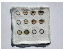
Fig. 1. Cotton textiles after different conditions of irradiation. Upper row (from left to right): 10 pulses at 1400 mJ/cm 2 , 50 pulses at 1400 mJ/cm 2 , 200 pulses at 1400 mJ/cm 2 , 500 pulses at 1400 mJ/cm 2 . Middle row (from left to right): 10 pulses at 1000 mJ/cm 2 , 50 pulses at 1000 mJ/cm 2 , 200 pulses at 1000 mJ/cm 2 , 500 pulses at 1000 mJ/cm 2 . Lower row (from left to right): 2000 pulses at 80 mJ/cm 2 , 5000 pulses at 80 mJ/cm 2 .
