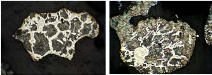
Fig. 6. Microstructure of the dispersed particles of reduced scale by graphite at 1150°C, 60 min isothermal retention fraction 0,63mm, etched with nital 100X
