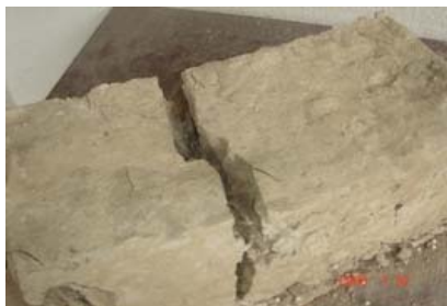
Fig. 2. Pure clay brick, cracked after drying and the shrinkage results
