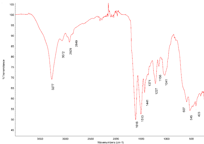
Fig. 11. Typical FTIR spectra for un-dyed silk fiber
