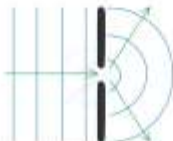
Diffraction: when a wave passes through a narrow gap, it spreads out.
