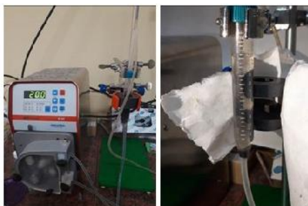
Figure 1. Experimental model for the vertical magnetic separator: a) elementary b) elementary with two individual separation zones
